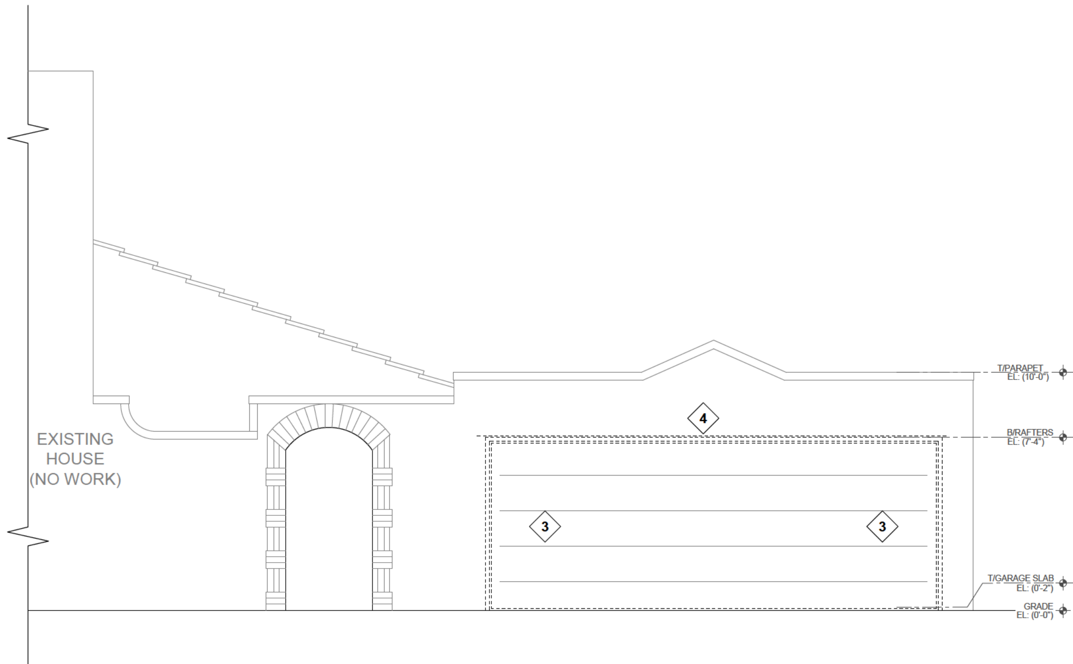
DEMOLITION NORTHWEST ELEVATION SCALE: 1/4" = 1'-0"
