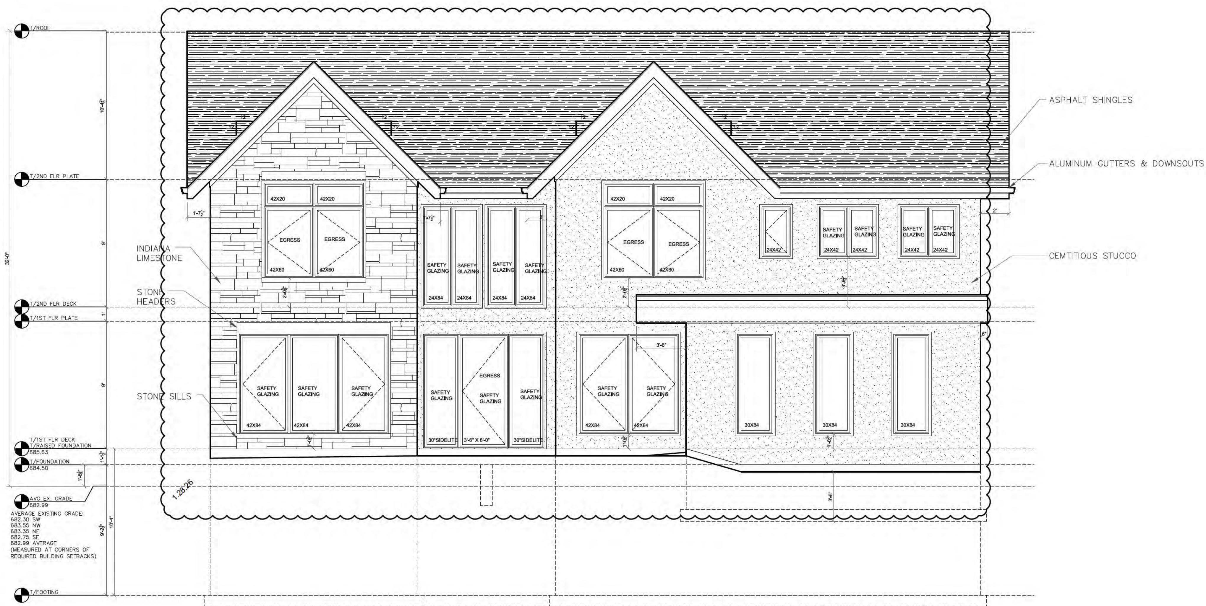
01 WEST (FRONT) ELEVATION SCALE: 1/4"=1'-0"
