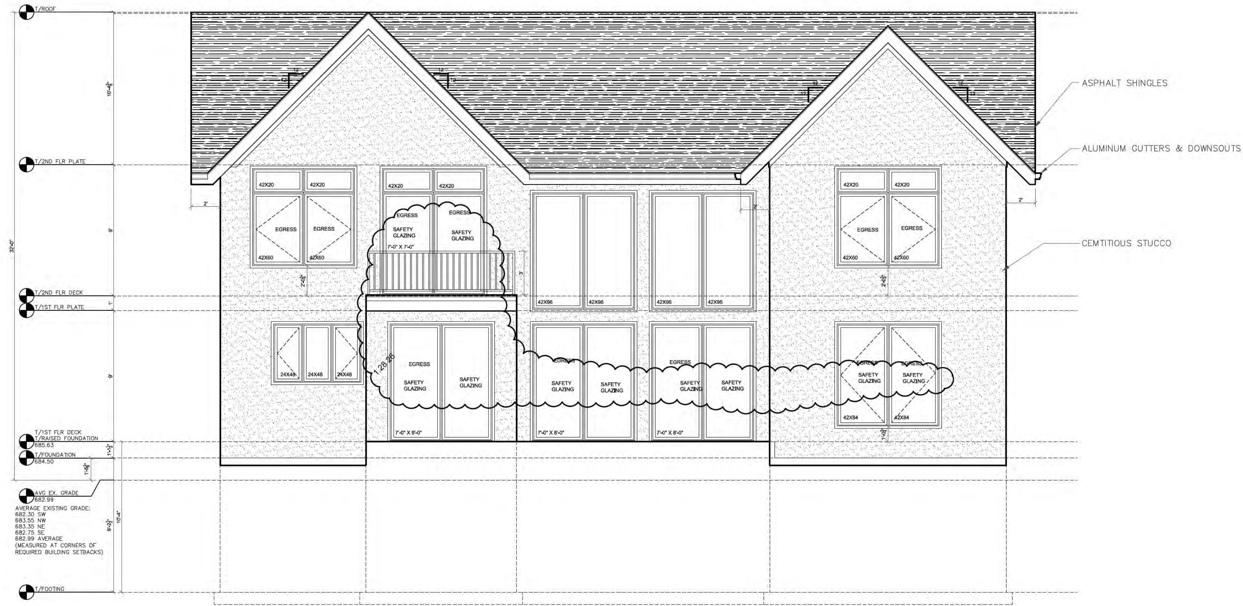
01 WEST (FRONT) ELEVATION SCALE: 1/4"=1'-0"
