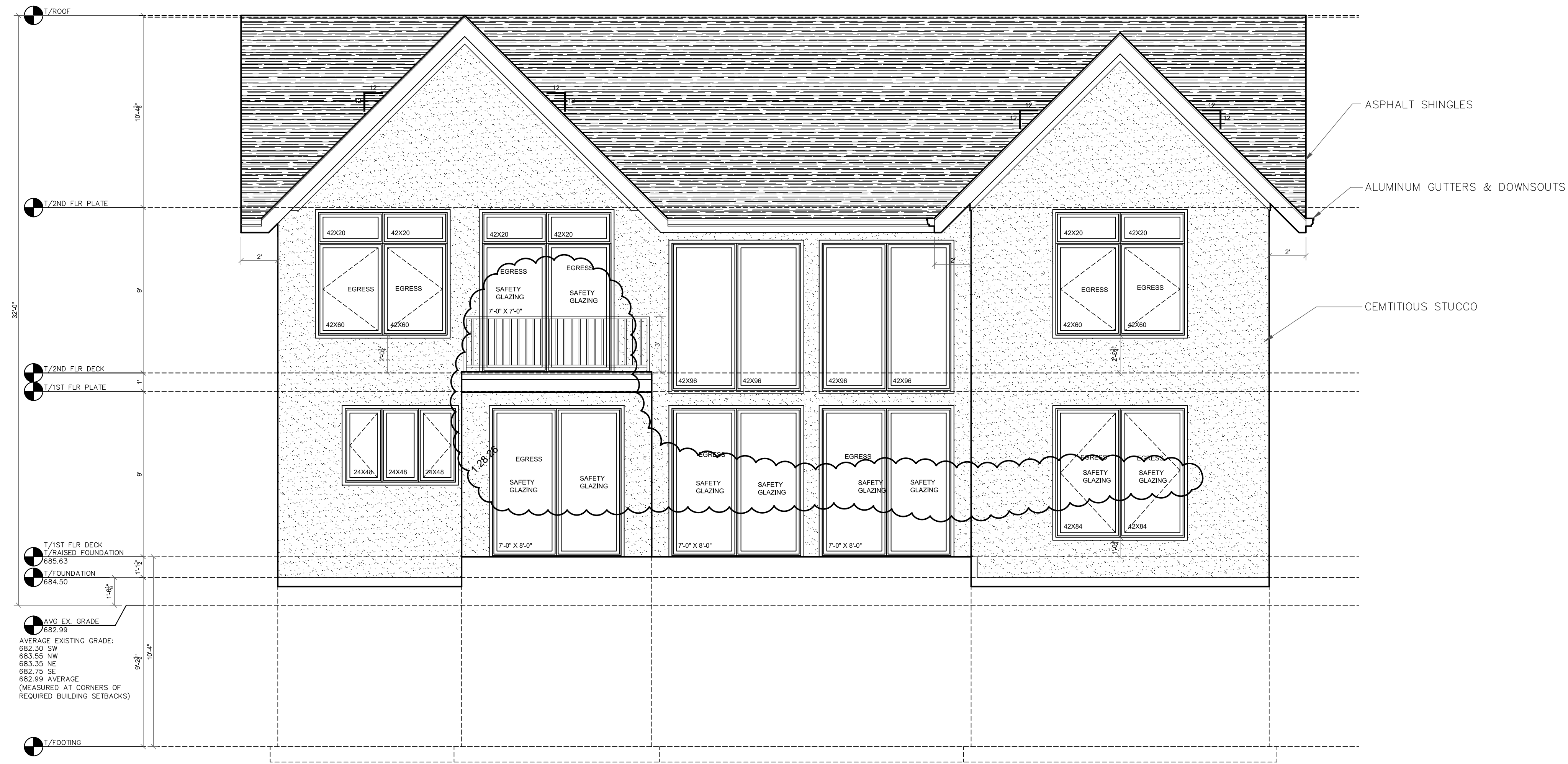
01 WEST (FRONT) ELEVATION SCALE: 1/4"=1'-0"
