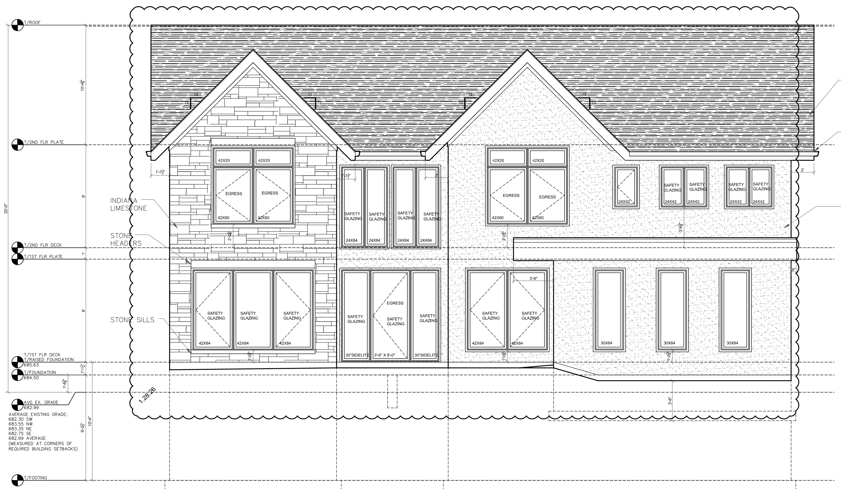
01 WEST (FRONT) ELEVATION SCALE: 1/4"=1'-0"
